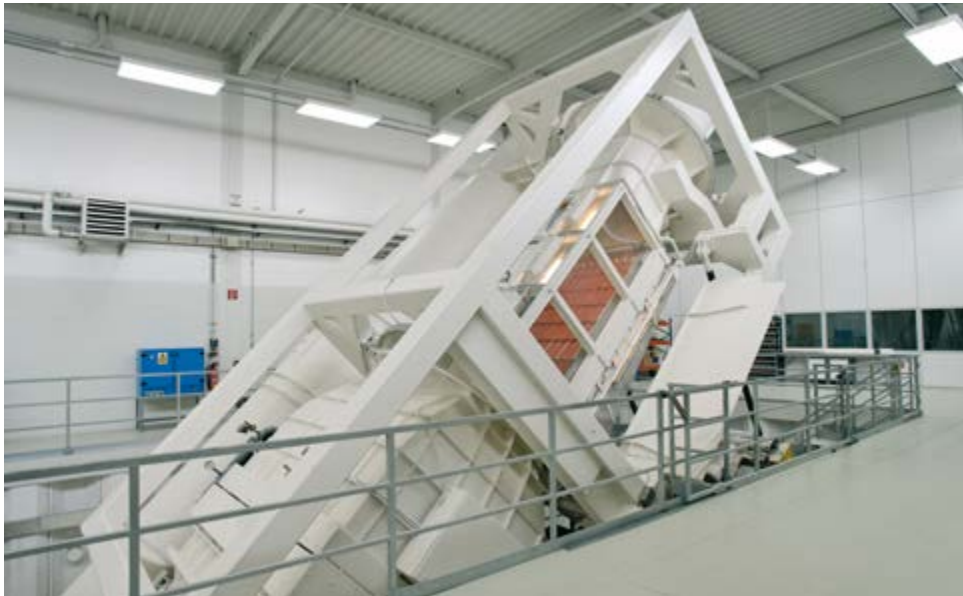
Wind tunnel testing area simulating heavy weather conditions at our Technical Centre in Heusenstamm.
